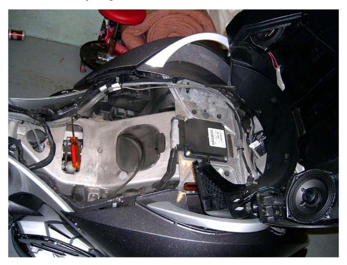
Don't forget to remove these two screws:
