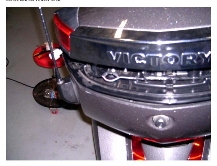
Once I cut the green/pink wire going to the left light I put a male connector on the side going to the light and female connector on both the new wire and the end of the old wire so that I could return it to factory if I need to.
