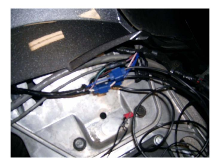
I tucked the controller in the trunk by the CB. I made everything nice and neat after this picture was taken. I also hooked up the ground wires to the bolt at the top left.
